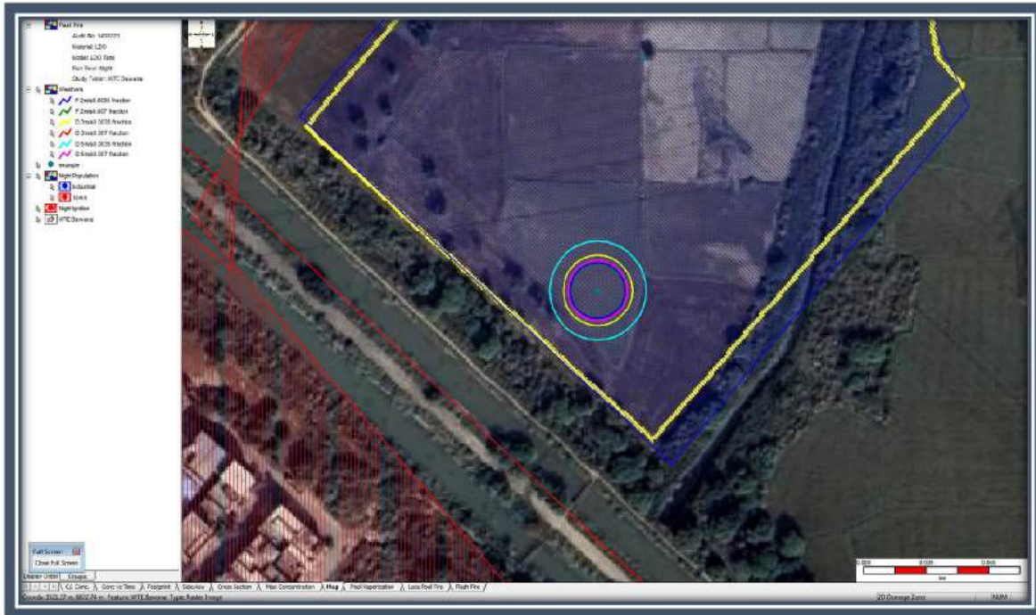
Fig. 7.5 Damage Contour for Flash Fire Scenario due to rupture at LDO Tank
