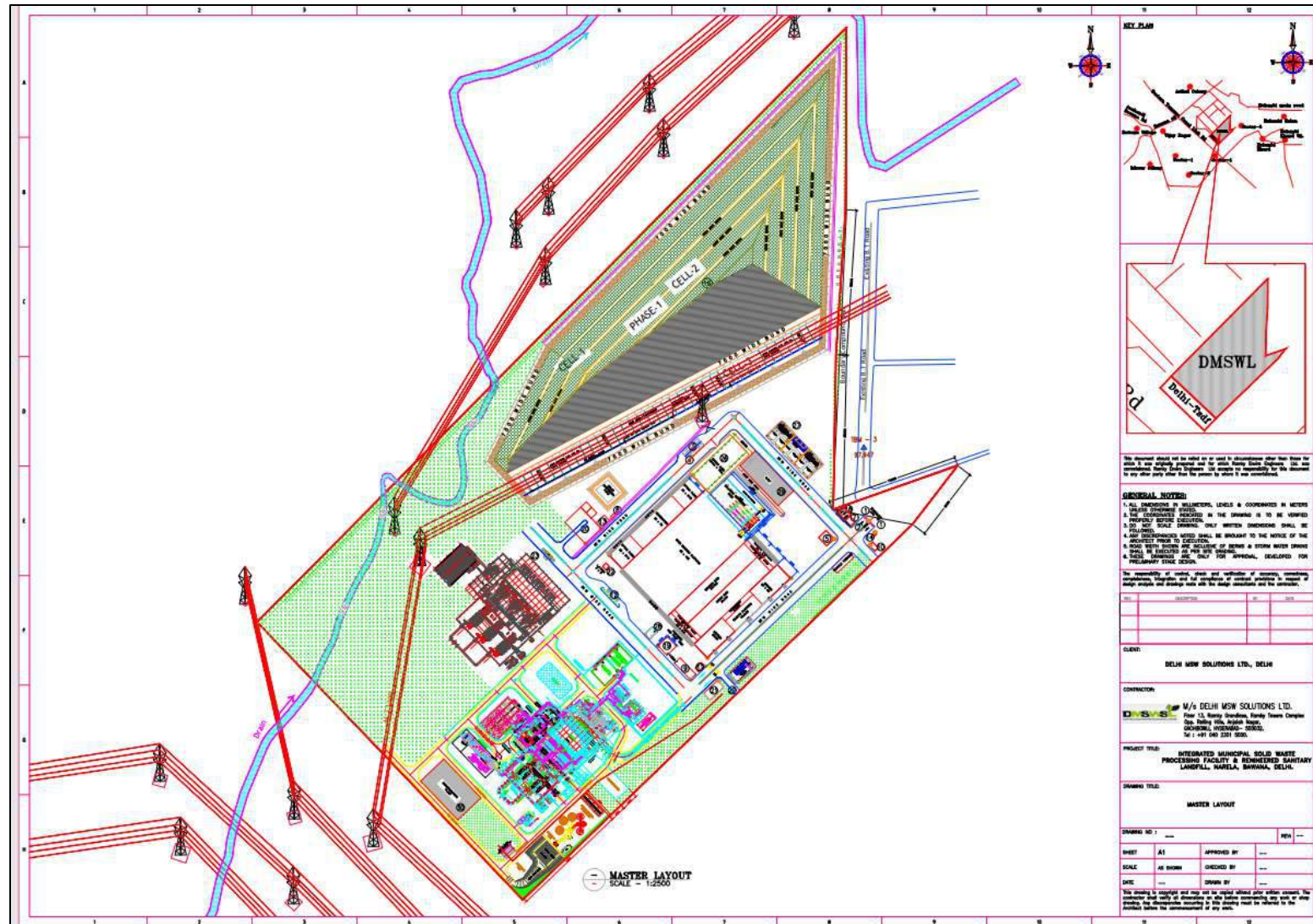
Figure 2.5: Layout of waste to energy plant
