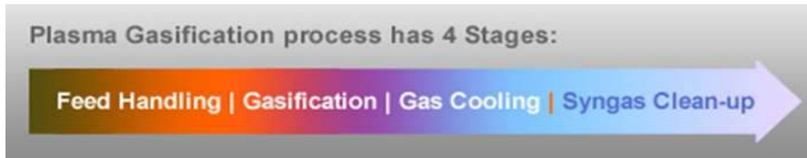
Figure 5.2 Flow Diagram of Process Stages of Plasma Arc Gasifier
