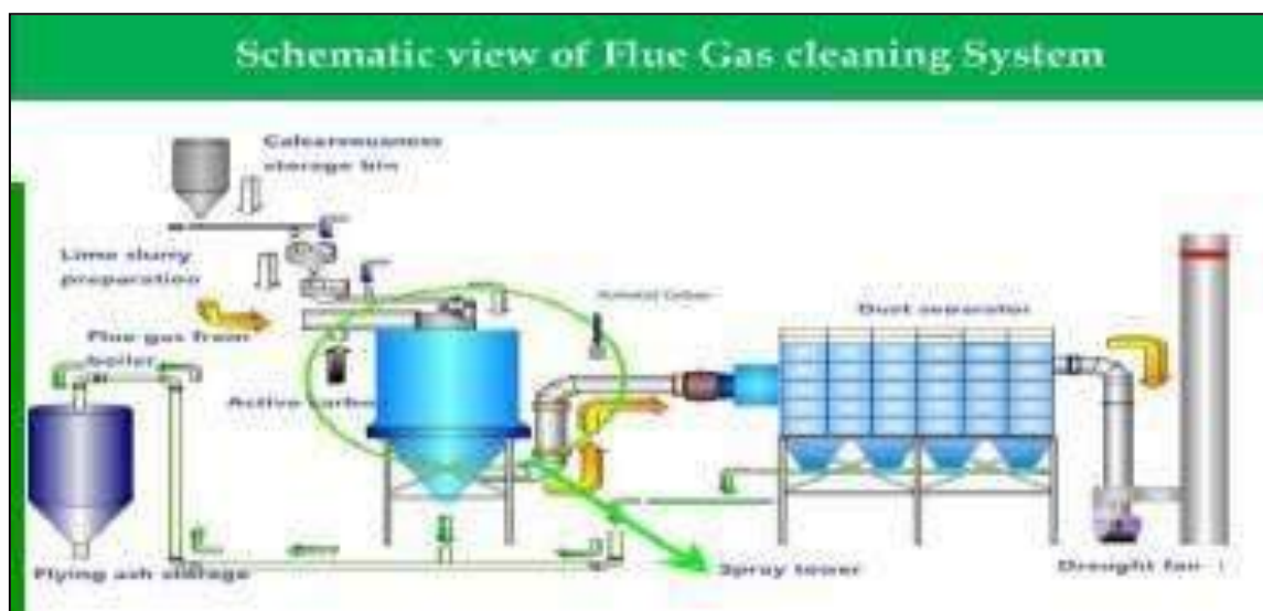
Figure 4.5: Schematic view of flue gas cleaning system
