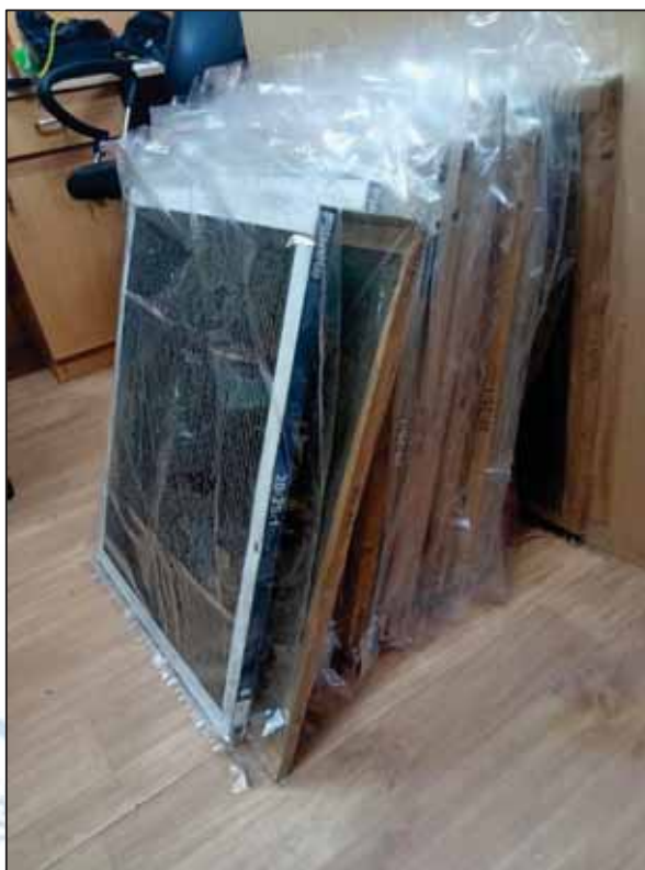
Figure 169. Saturated pre and fine filter sample.
