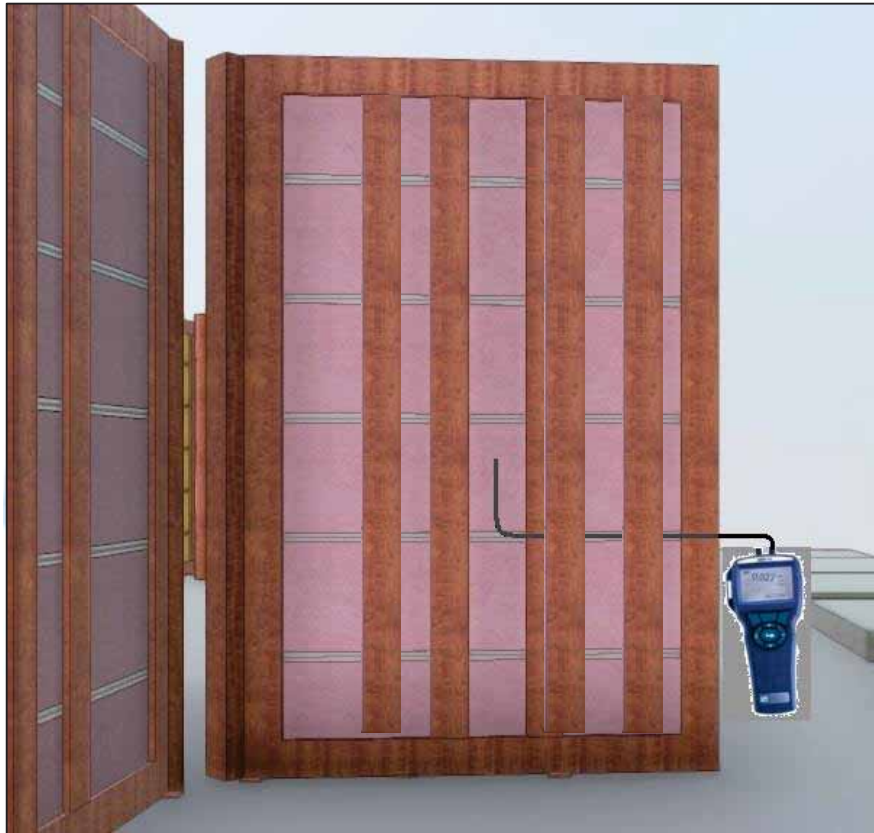
Figure 142. Side view showing the height of the location of the end of neoprene rubber tube of setup for measuring the static pressure drop across filter bank.
