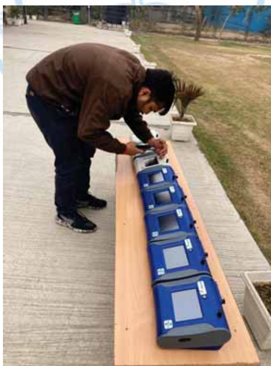
Figure 29. Colocation of the DustTrak and OPS.
