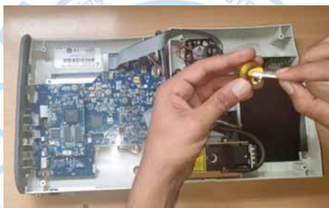
Figure 25. Internal cleaning of OPS.
